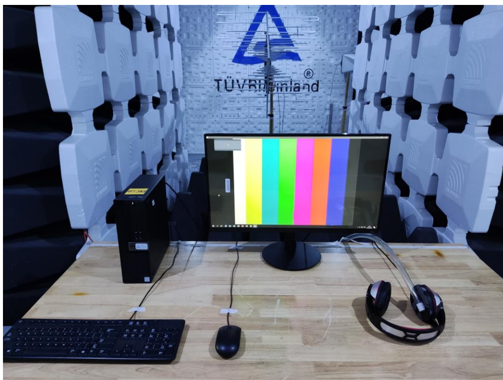
Photograph 4: Set-up for Radio-frequency Electromagnetic Field Amplitude Modulated
