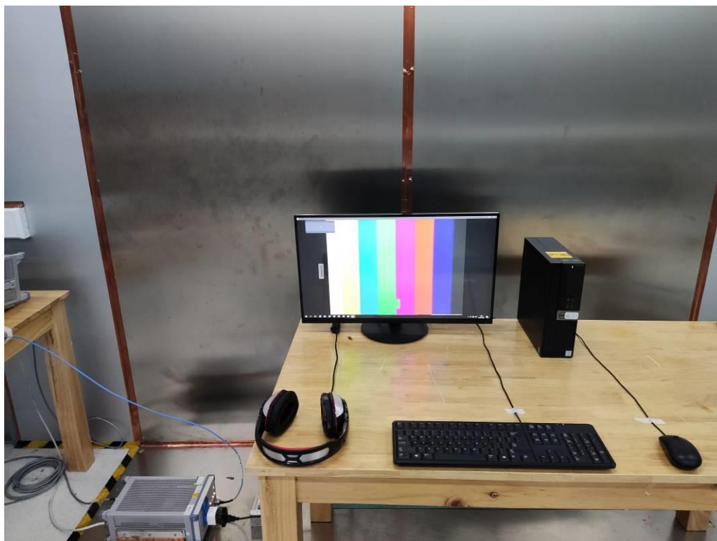
Photograph 2: Set-up for Radiated Emission(30MHz-1GHz)
