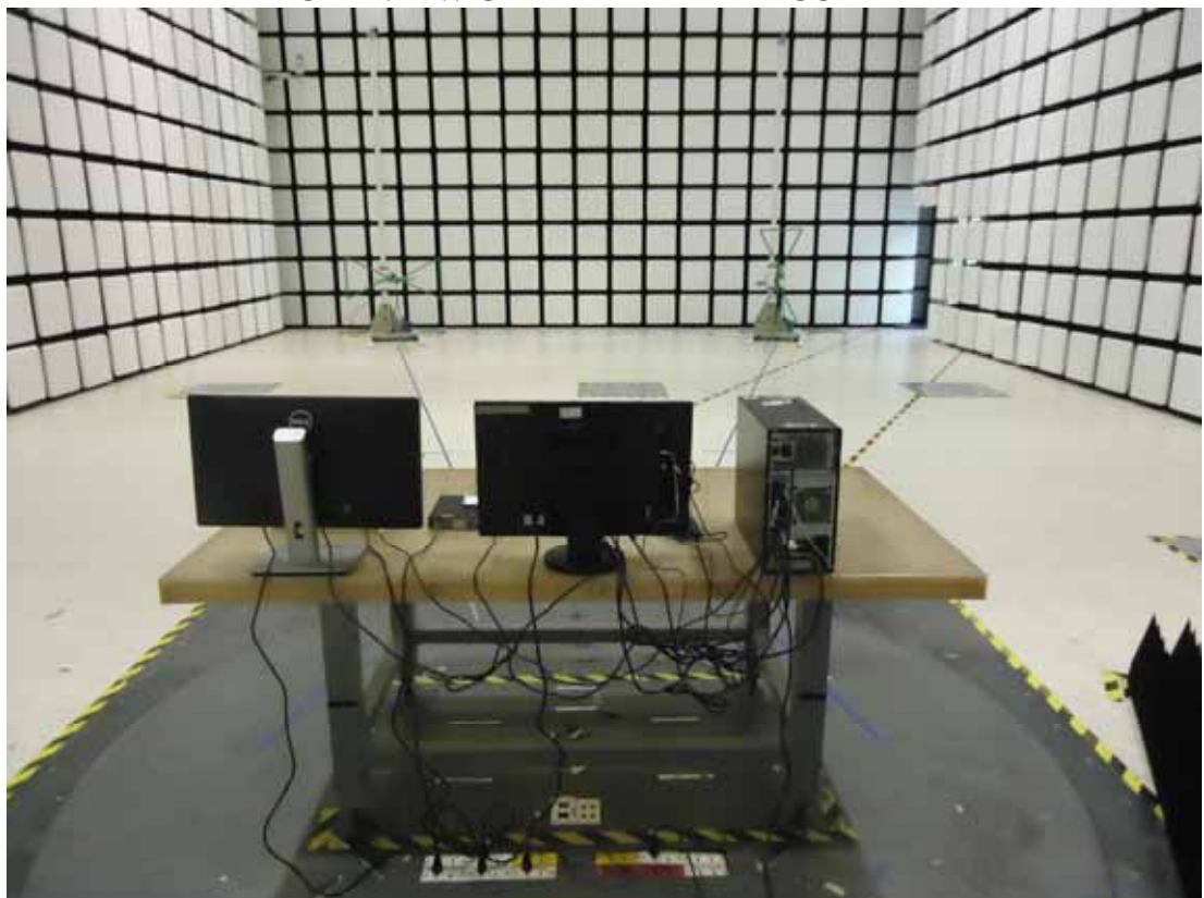
BACK VIEW OF RADIATED MEASUREMENT
