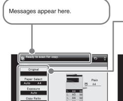
Settings appear here. If you press the  $\bigcirc$  key when the selection frame is on the bottom setting, the next screen will appear.
