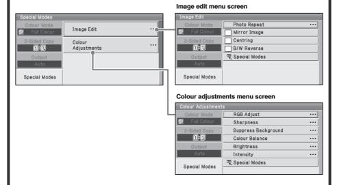
When you select a special mode with a checkbox ( $\square$ ), the checkbox changes to  $\checkmark$  and the setting is completed.
