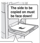
Load the paper in the horizontal orientation.
