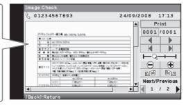
Example: The image check screen for a received fax
