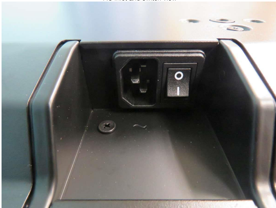
AC inlet and switch view
