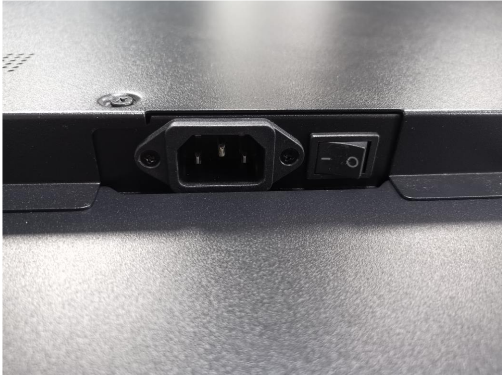
Figure 5. AC inlet view
