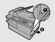
**2** Press the center roller with your finger to make it rotate a half turn back into the machine.
