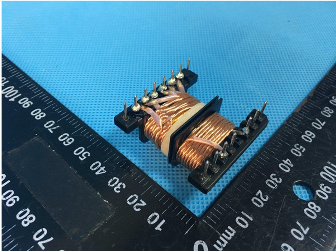
Photo 27 Transformer THA1 view
