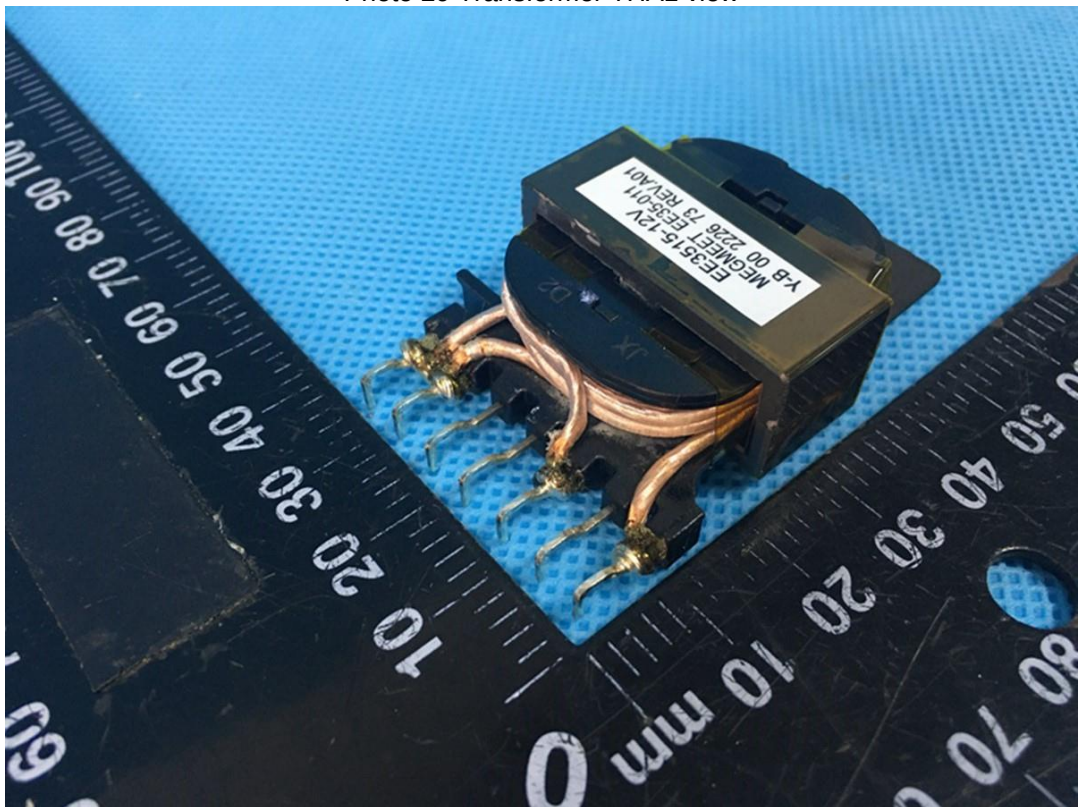
Photo 30 Transformer TH1 view
