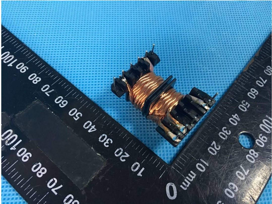
Photo 29 Transformer TH2/TH3 view
