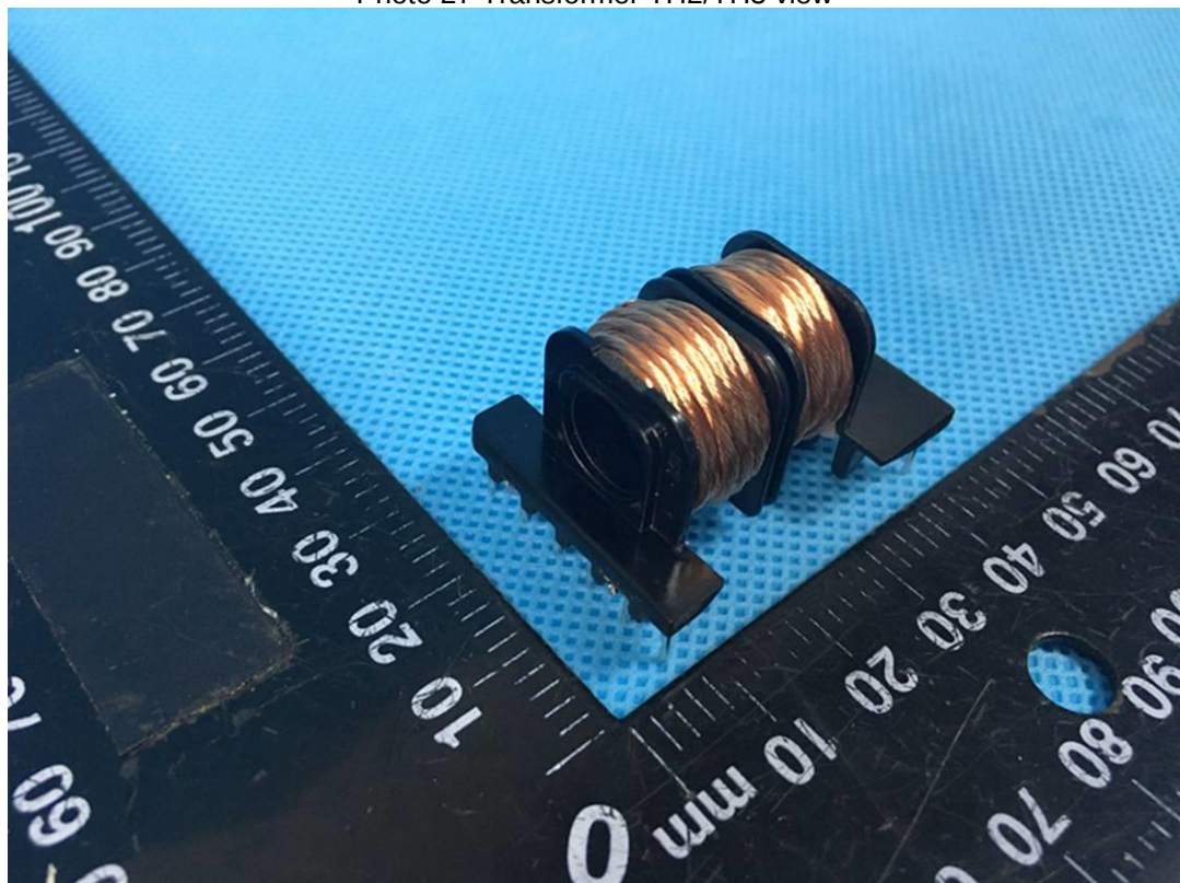
Photo 28 Transformer TH2/TH3 view
