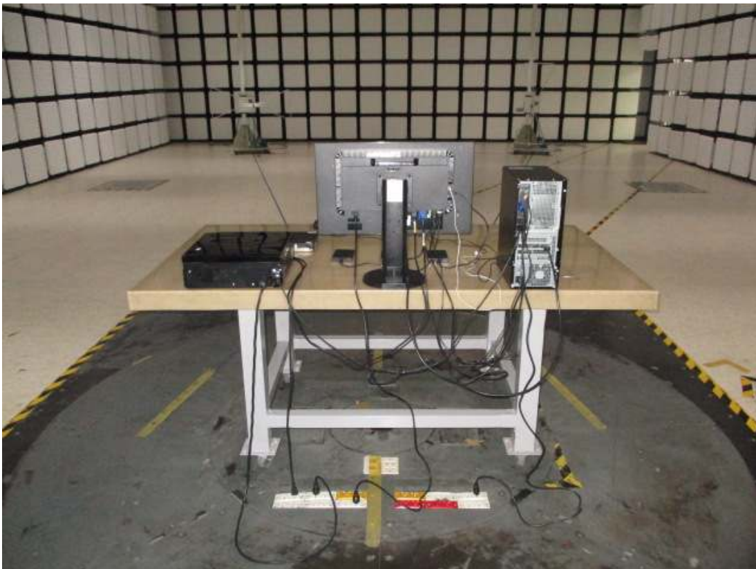
Back View of Radiated Measurement
