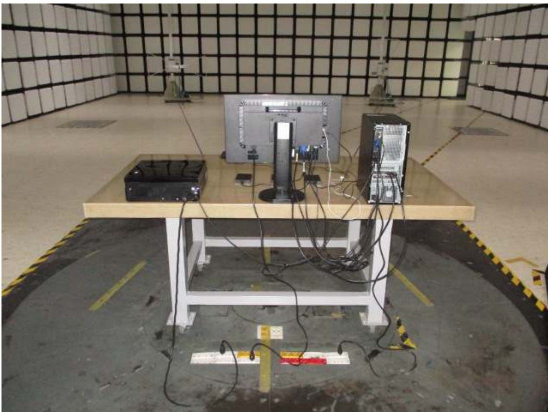
Back View of Radiated Measurement
