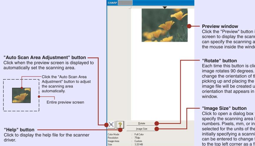
Click the "Preview" button in the Set-up screen to display the scanned image. You can specify the scanning area by dragging the mouse inside the window.
