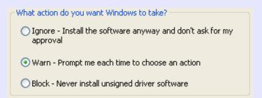
If the option "Block" has been selected for your computer, then the MFP driver will not be installable. Select the option "Warn" and then install the MFP driver as explained in "INSTALLING THE SOFTWARE" in the Operation Manual.
