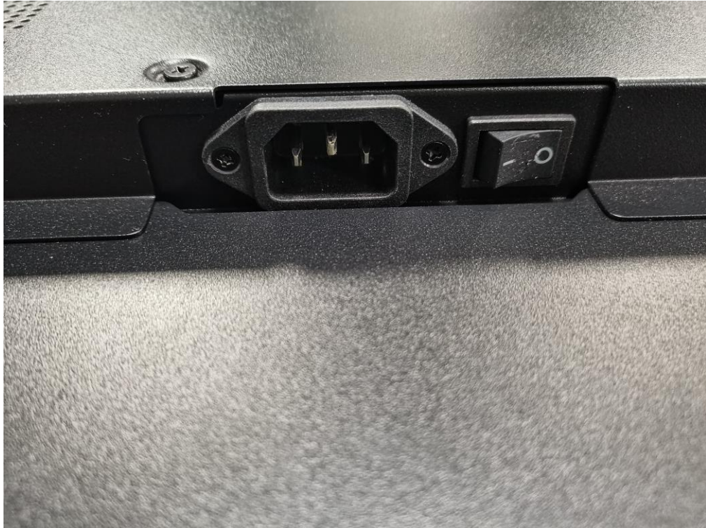
Figure 5. AC inlet view
