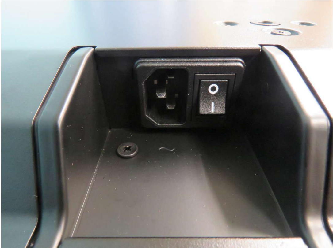
AC inlet and switch view
