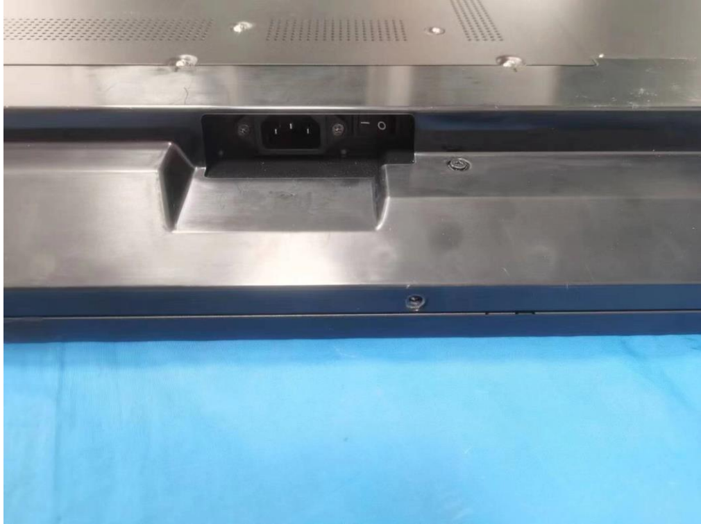
Figure 5 AC inlet view
