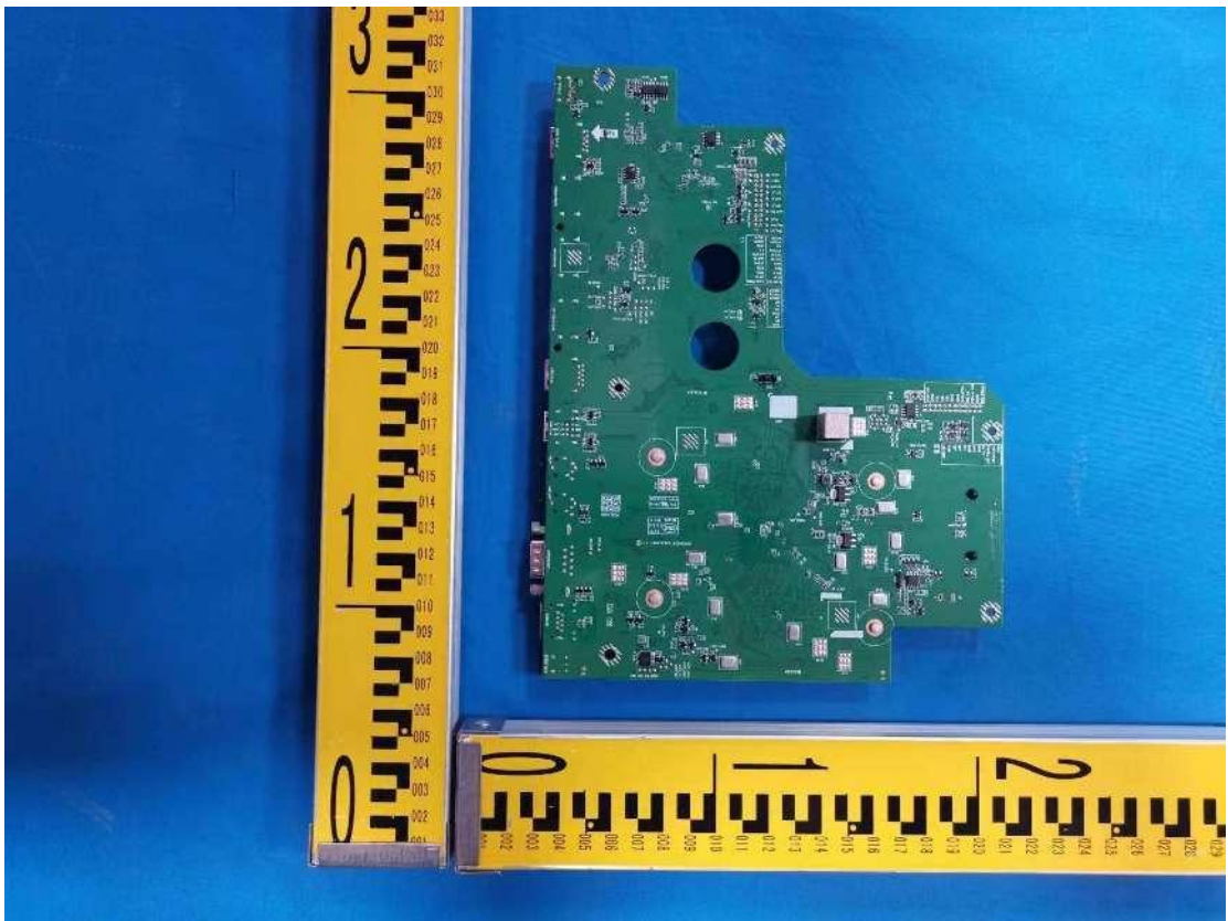
Figure 15. Main board T.MT9666.71 solder side view
