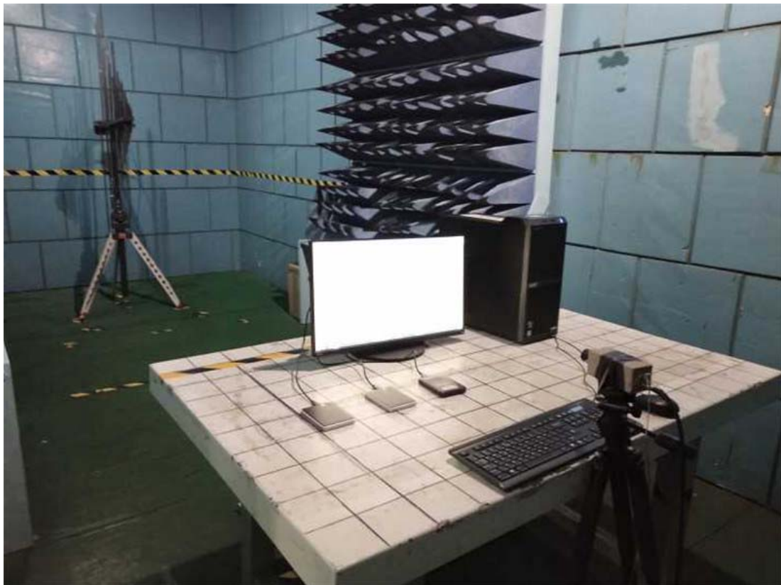
15.5. Photo of RF Strength Susceptibility Test
