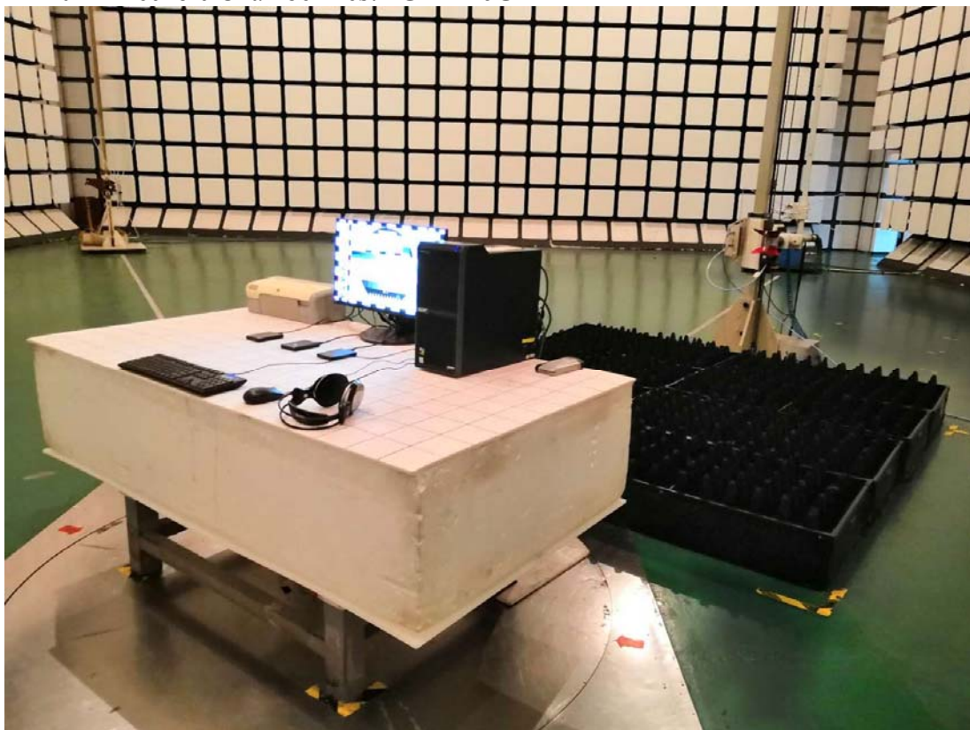
In 10m Anechoic Chamber Test 1GHz – 6GHz
