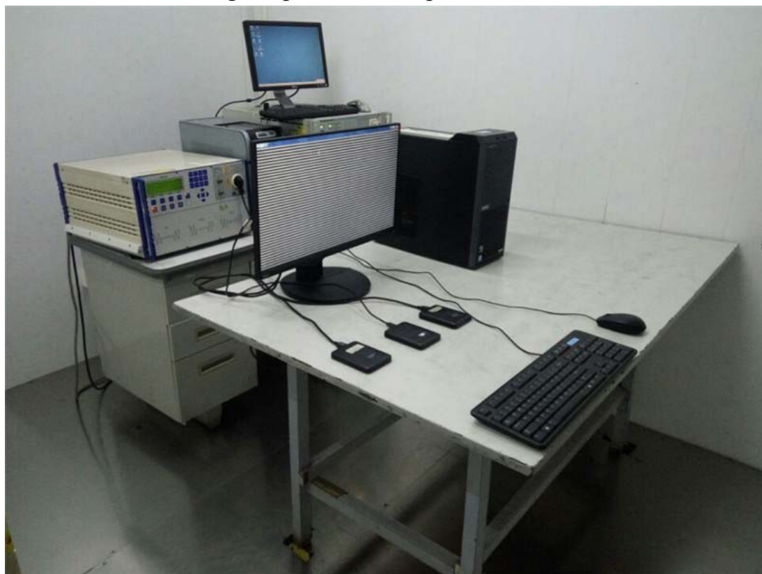
15.10. Photo of Voltage Dips and interruptions test
