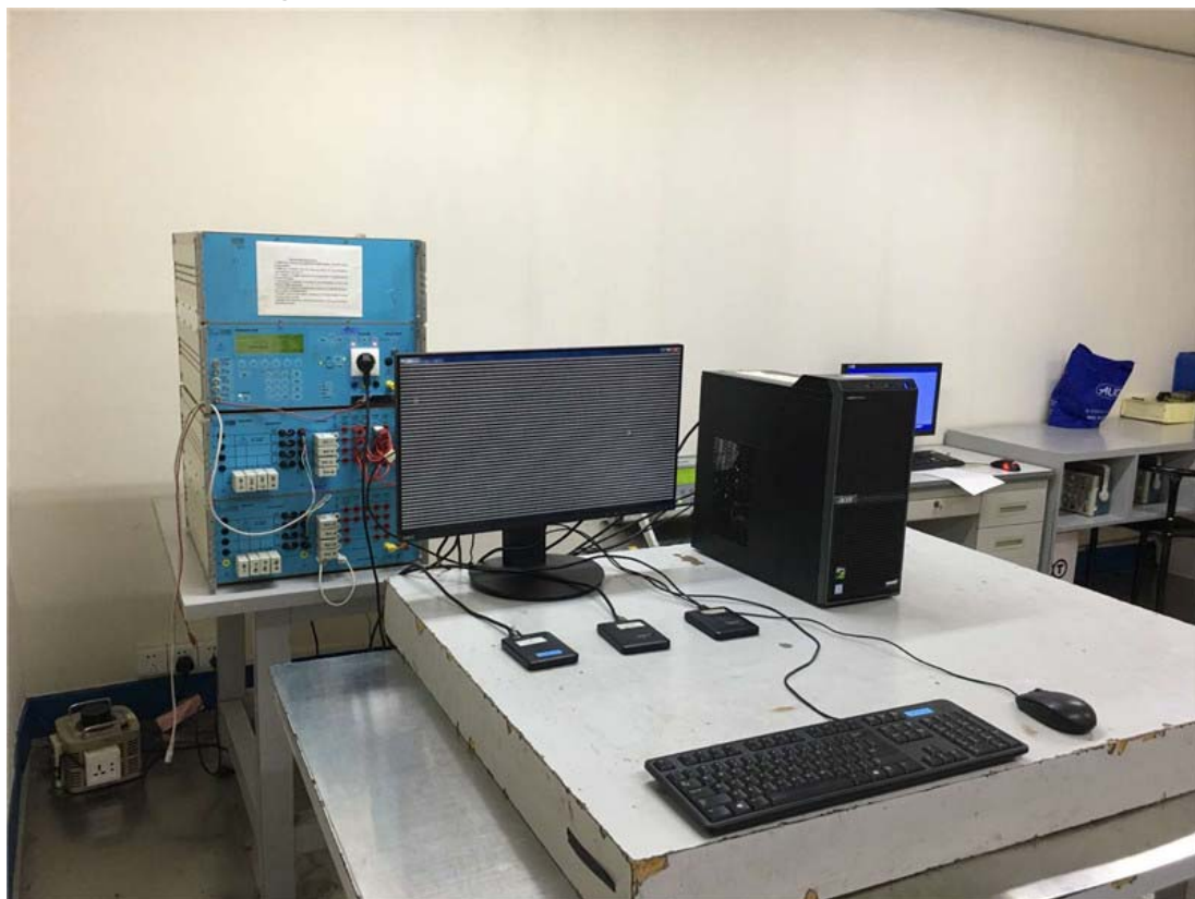
15.7.Photo of Surge Test
