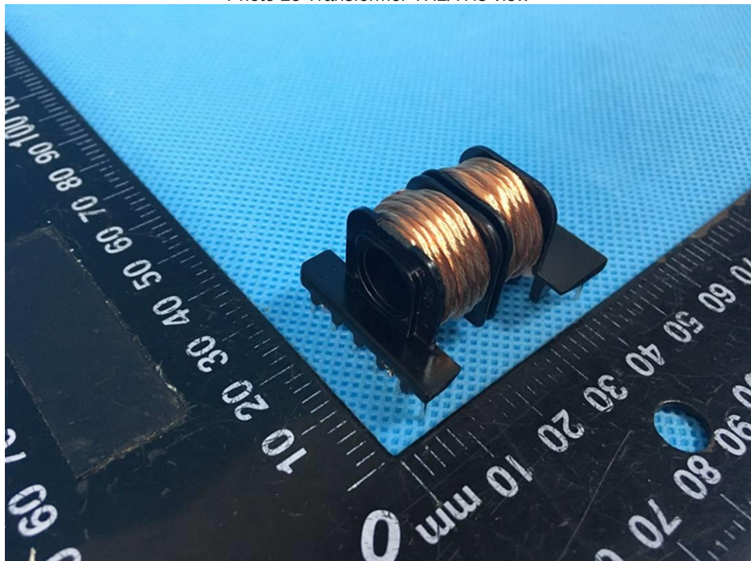
Photo 26 Transformer TH2/TH3 view
