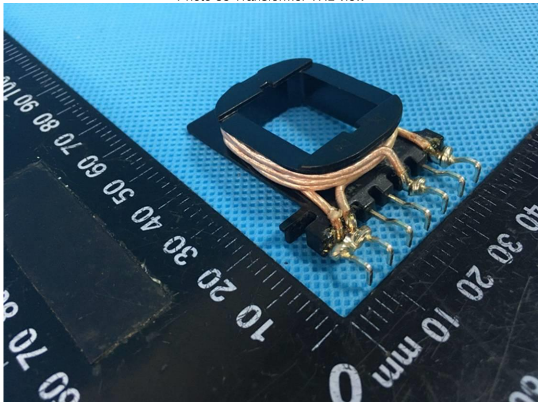
Photo 36 Transformer TH1 view
