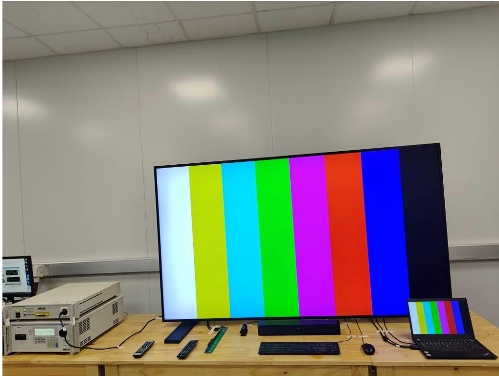
Photograph 9: Set-up for Harmonics & Flicker
