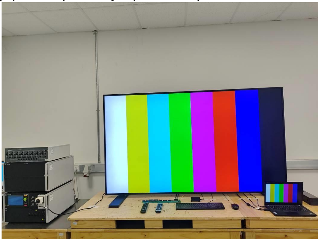
Photograph 8: Set-up for Voltage Dips and Interruptions
