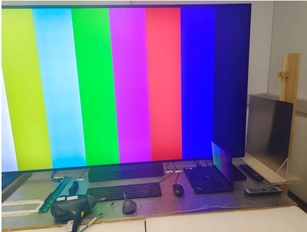
Photograph 7: Set-up for Electrostatic Discharges (ESD)
