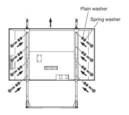
7 Confirm that the LCD Monitor is mounted securely, and then remove the hooks of the hoisting device.
