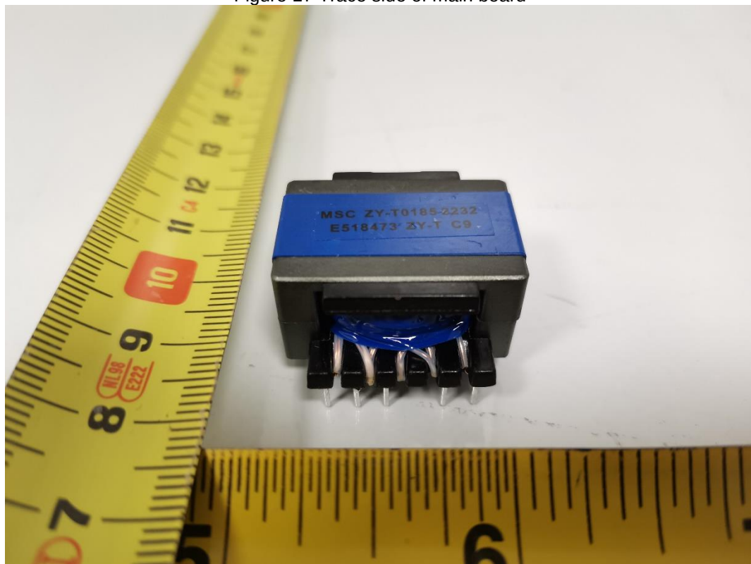
Figure 18 Transformer T1 view
