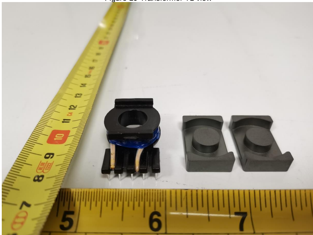
Figure 20 Transformer T1 view
