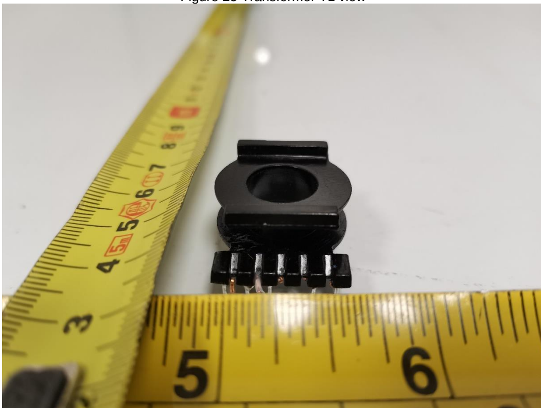
Figure 26 Transformer T1 view
