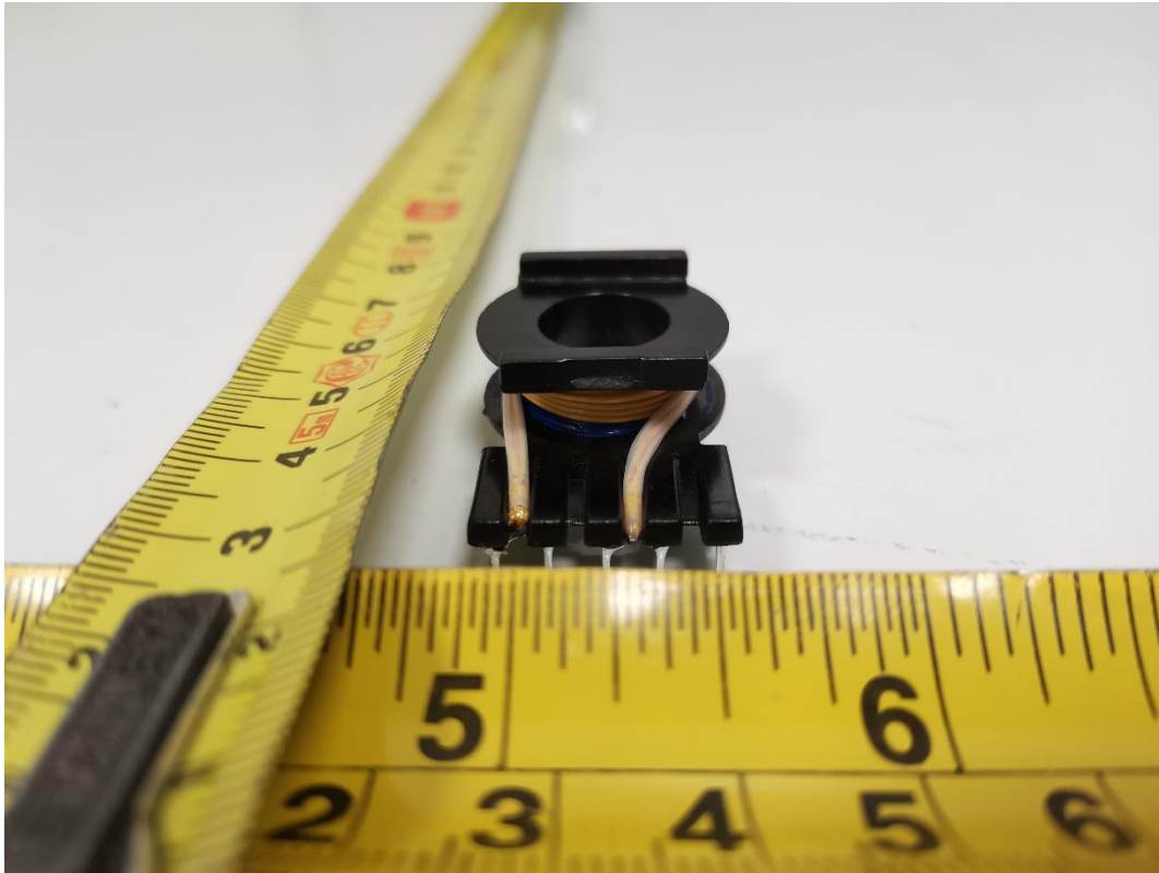
Figure 23 Transformer T1 view
