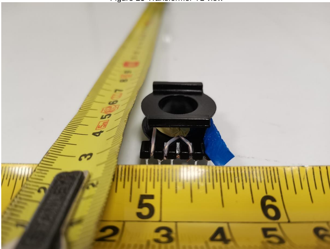
Figure 24 Transformer T1 view
