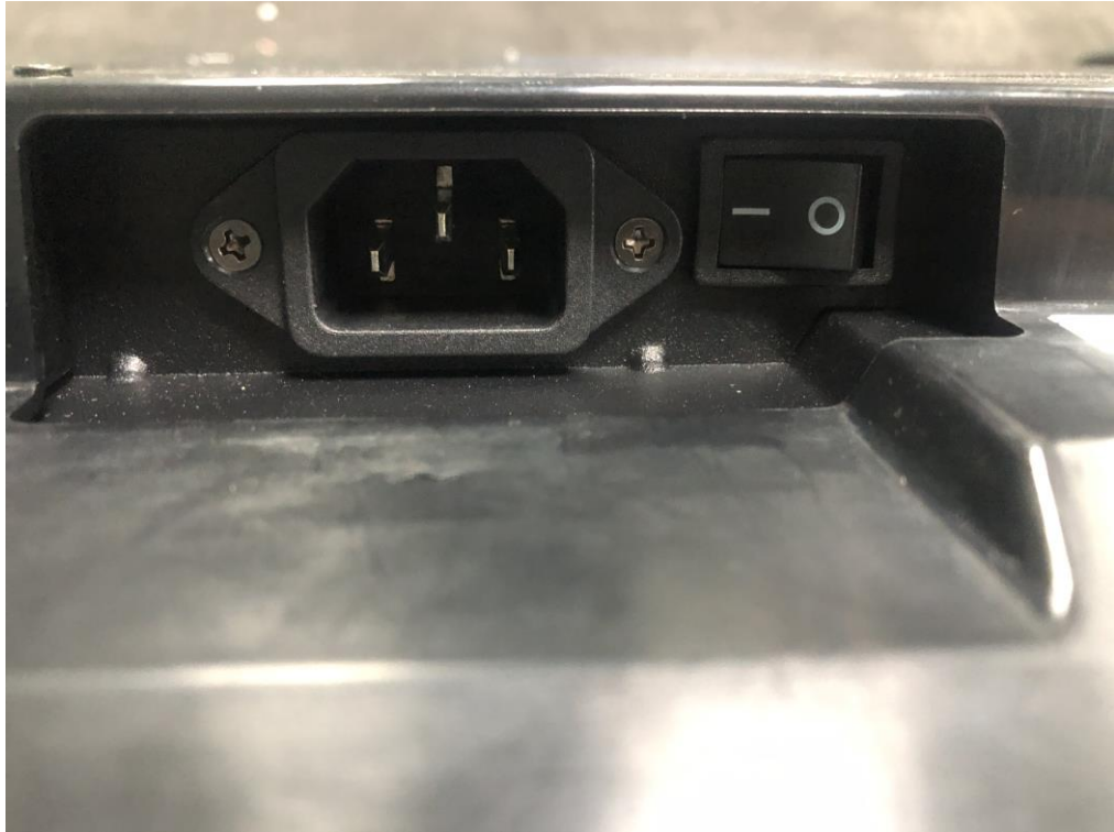
Figure 5 AC inlet view
