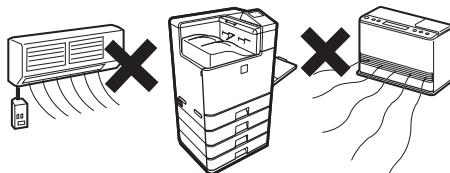
The paper will become damp and condensation may form inside the machine, causing misfeeds and dirty output.
