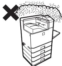
If dust enters the machine, dirty output and machine failure may result.
