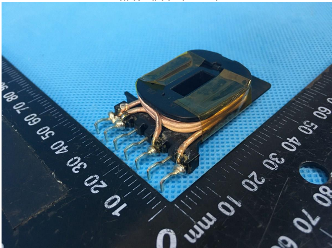
Photo 34 Transformer TH1 view
