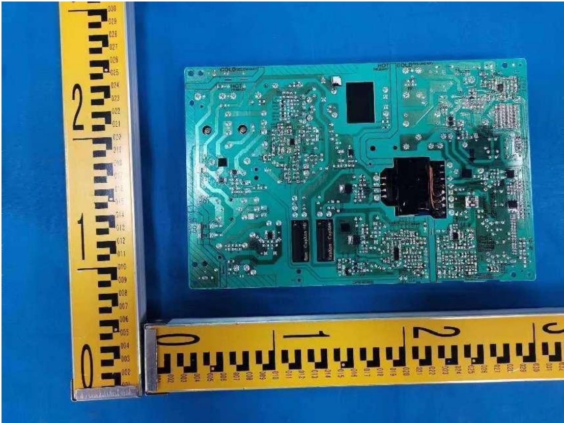
Figure 13. Power board PW.D232W2.751 solder side view
