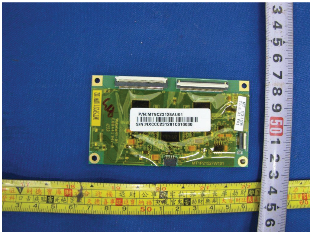
Figure 16. Touch-sensitive screen interfacing board MT1P21527W101
