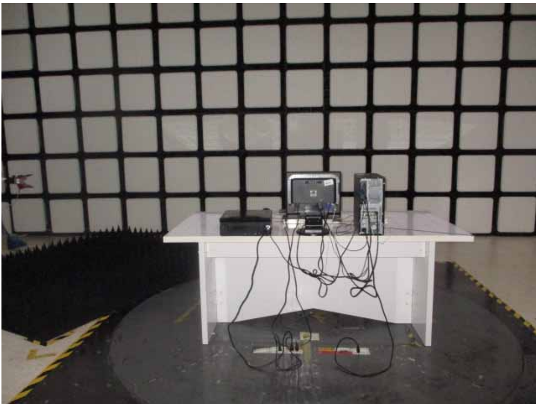
Back View of Radiated Measurement
