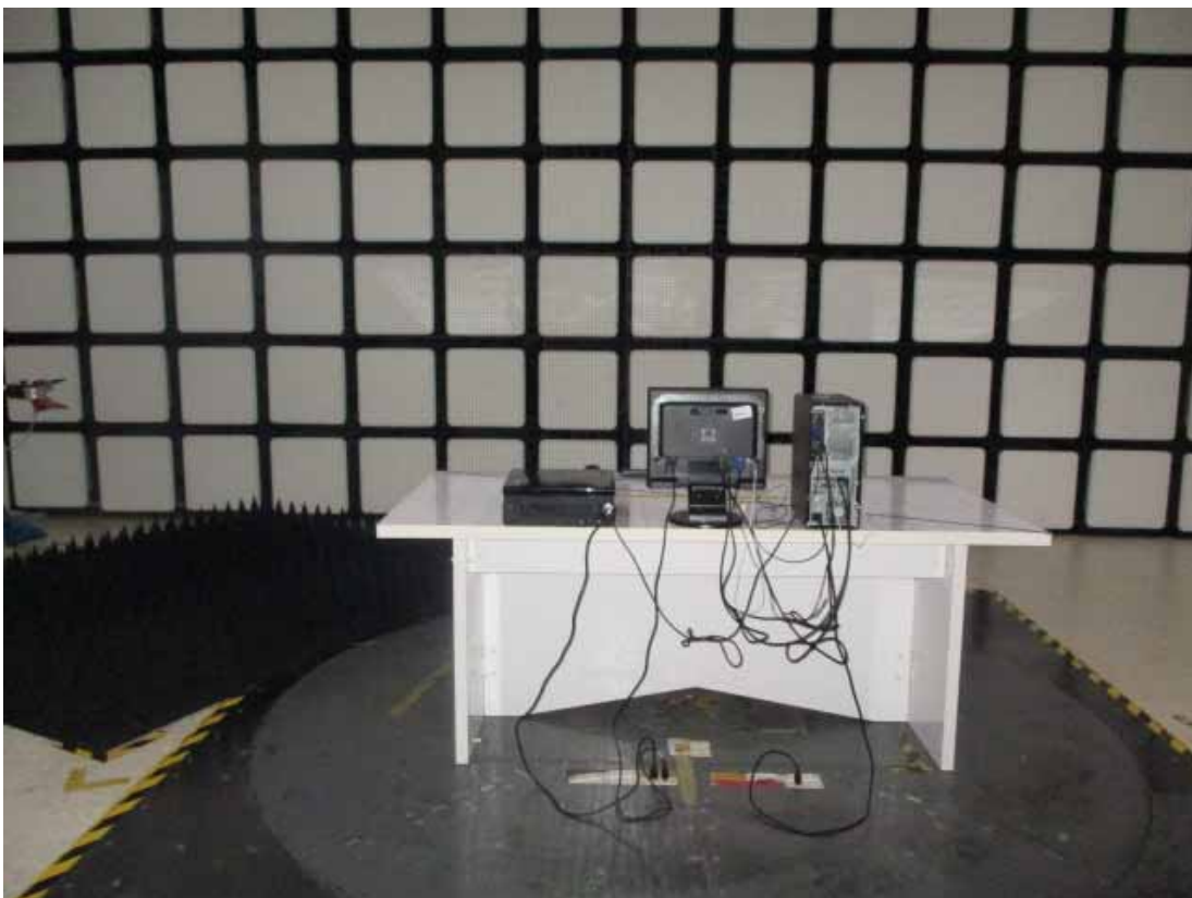
Back View of Radiated Measurement
