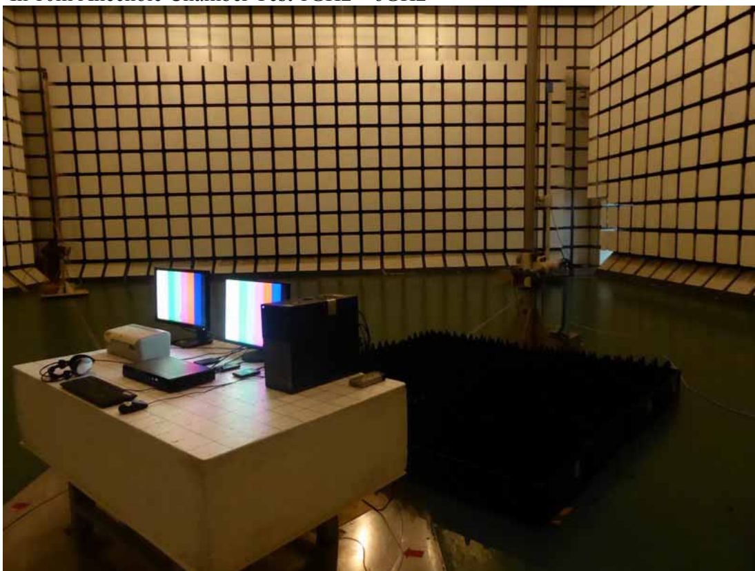
In 10m Anechoic Chamber Test 1GHz – 6GHz
