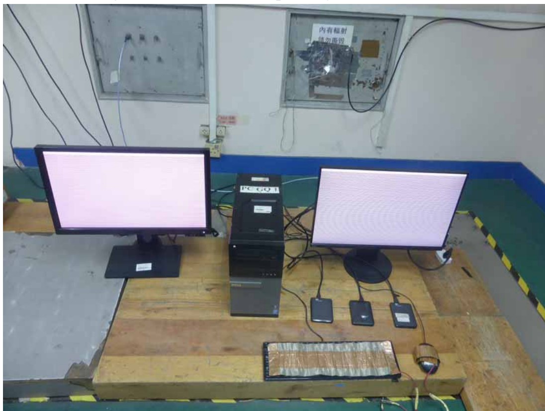
15.8.Photo of Injected Currents Susceptibility Test
