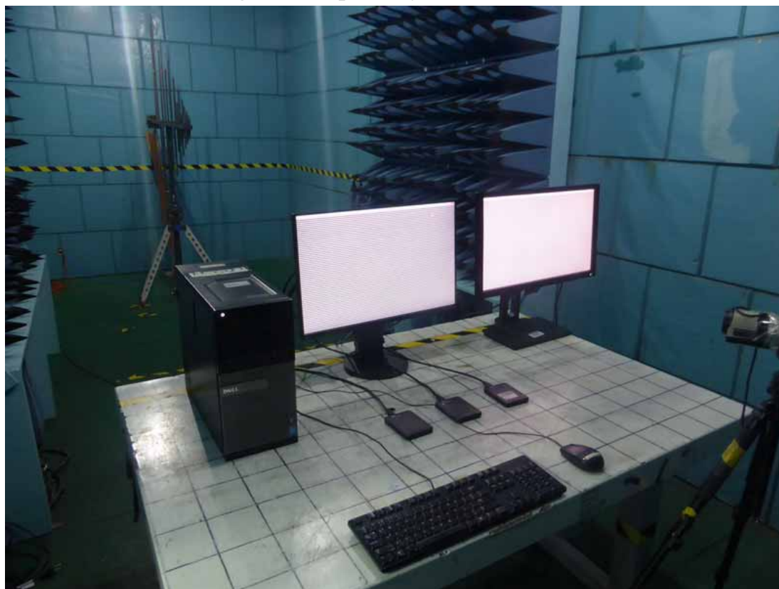
15.5.Photo of RF Strength Susceptibility Test
