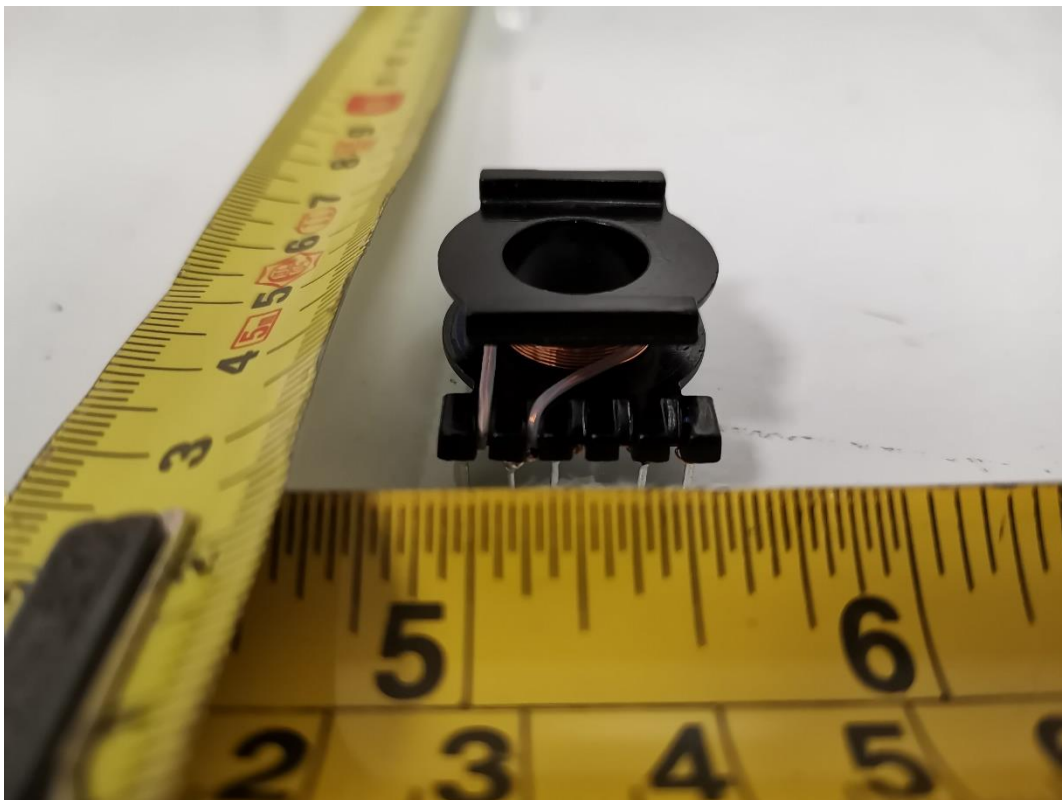
Figure 24. Transformer T1 view
