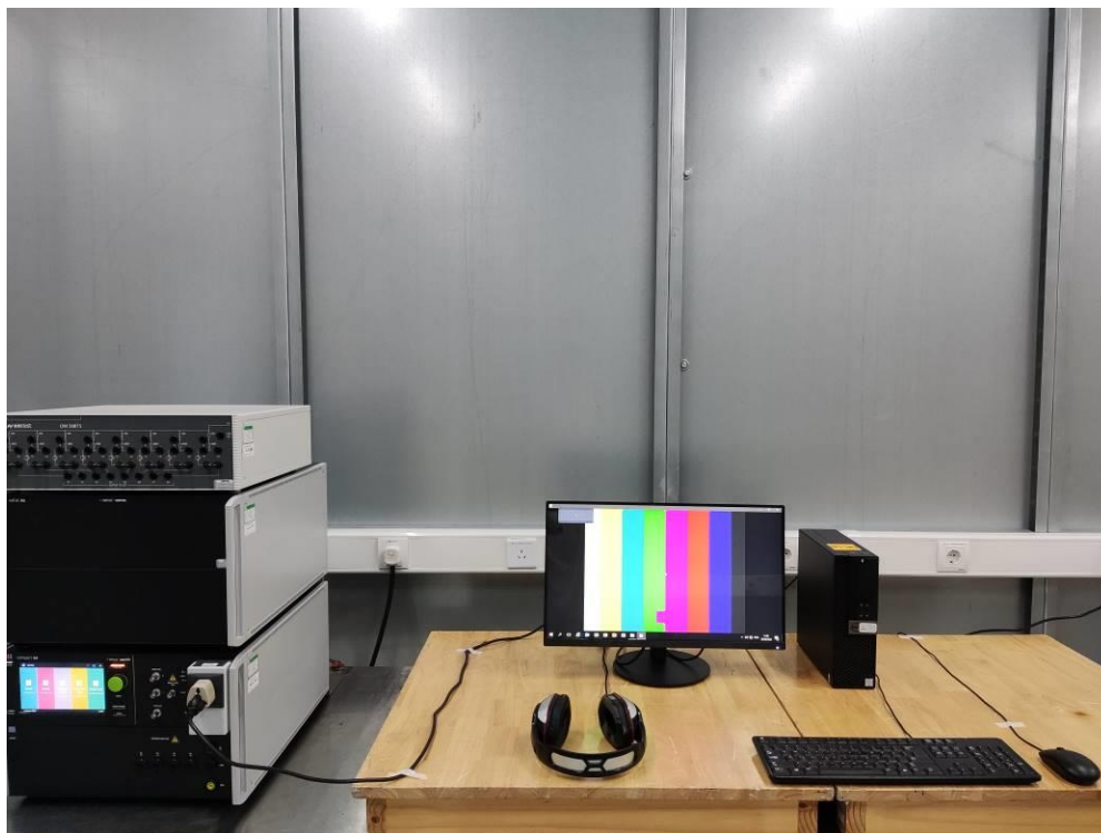
Photograph 8: Set-up for Voltage Dips on AC Mains
