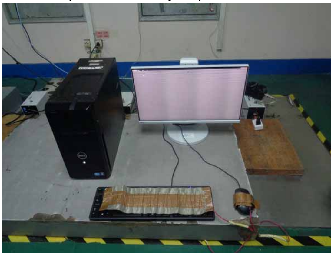
15.8.Photo of Injected Currents Susceptibility Test
