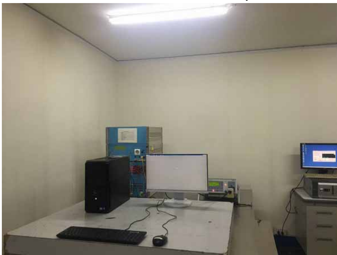
15.6.Photo of Electrical Fast Transient/Burst Immunity Test
