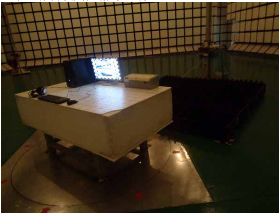
In 10m Anechoic Chamber Test 1GHz – 6GHz
