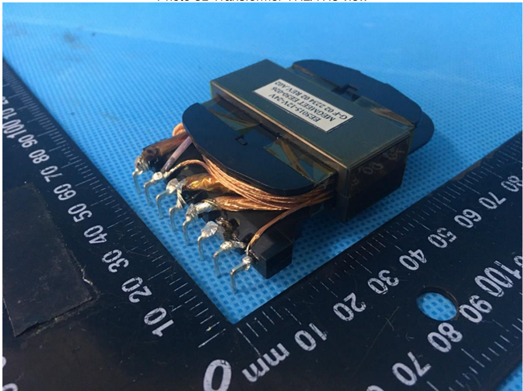
Photo 32 Transformer TH1 view
