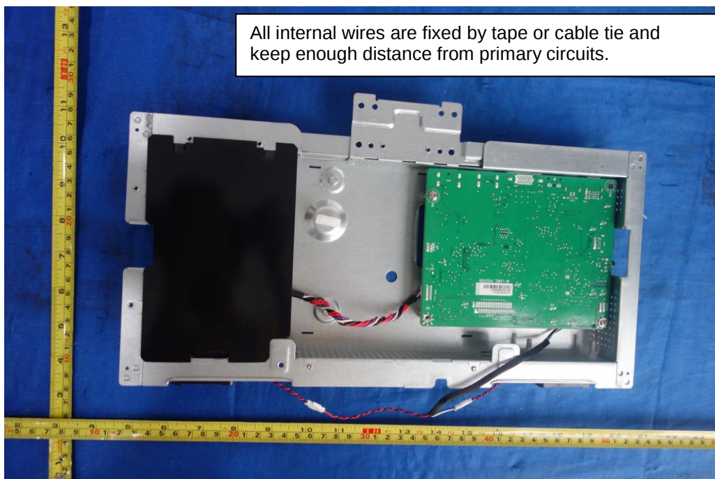
Figure 2. Internal view of metal enclosure type A
