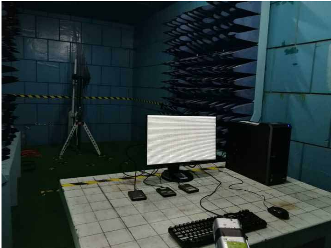
15.5.Photo of RF Strength Susceptibility Test
