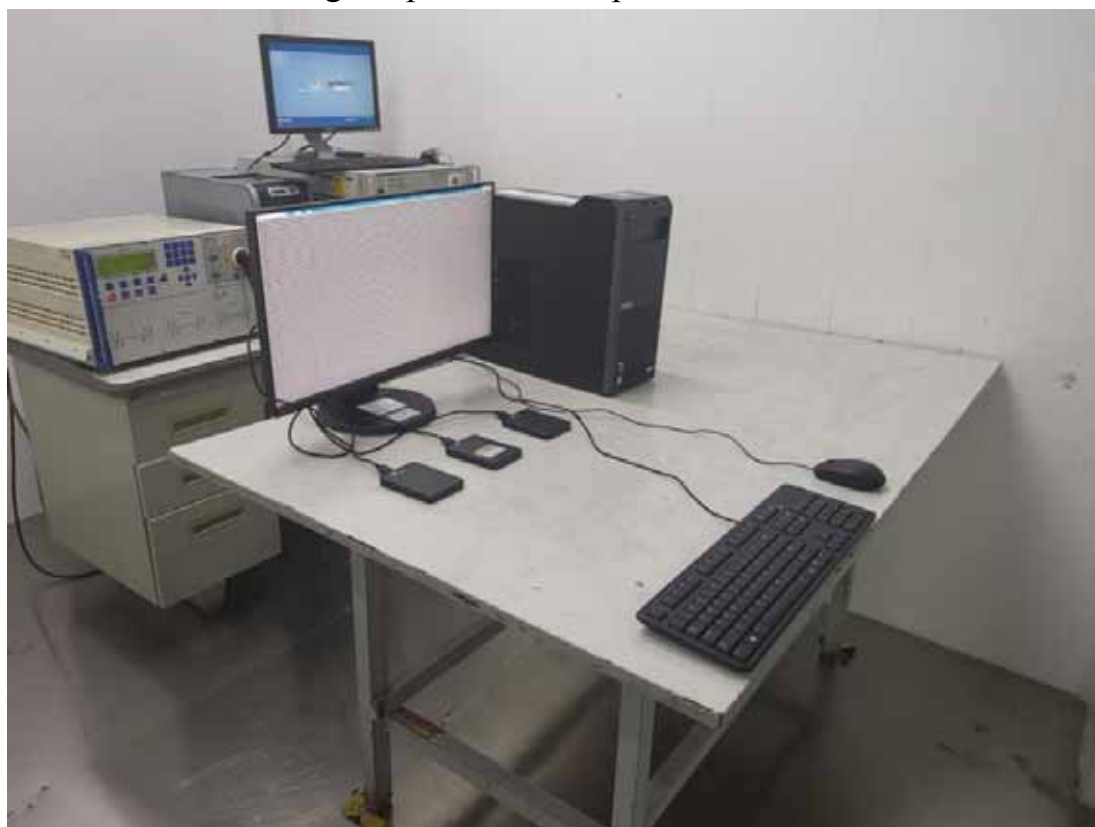
15.10. Photo of Voltage Dips and interruptions test
