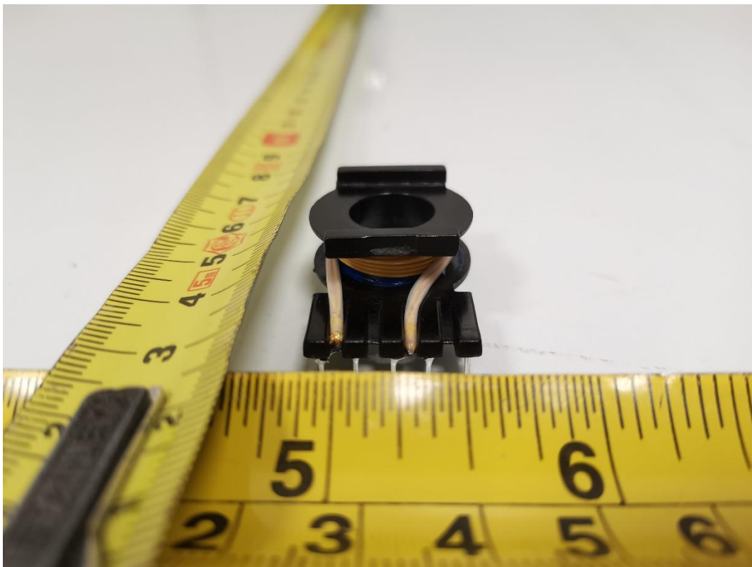
Figure 22. Transformer T1 view
