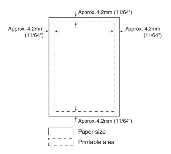
●The print area is the entire page excluding a margin of 4.2 mm (11/64") at each edge. The actual print area may vary depending on the printer driver used and the type of software application.
