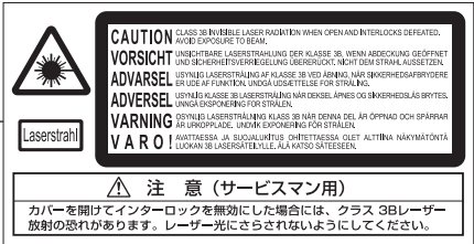
The above label is affixed to the laser unit inside the machine.
