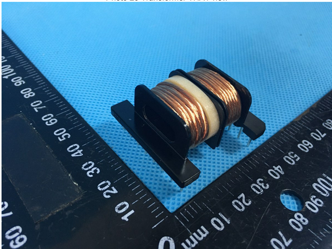
Photo 26 Transformer THA1 view
