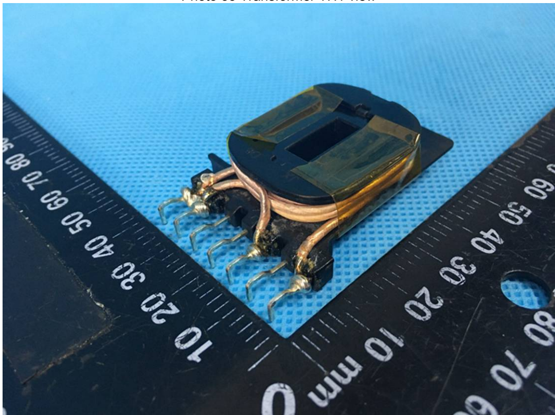
Photo 34 Transformer TH1 view
