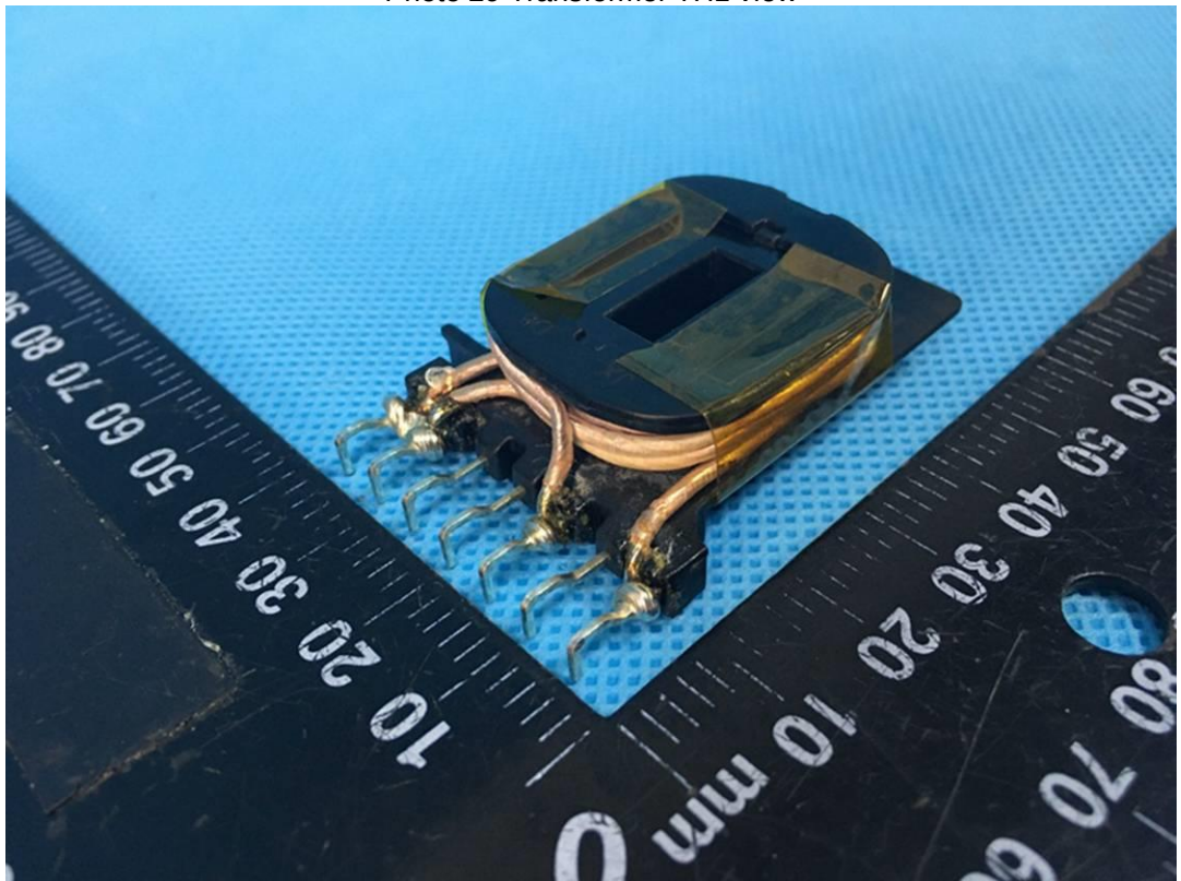
Photo 30 Transformer TH1 view
