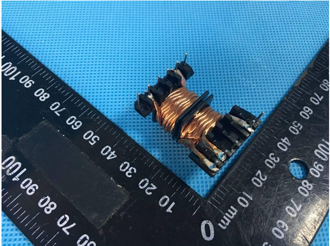
Photo 23 Transformer TH2/TH3 view
