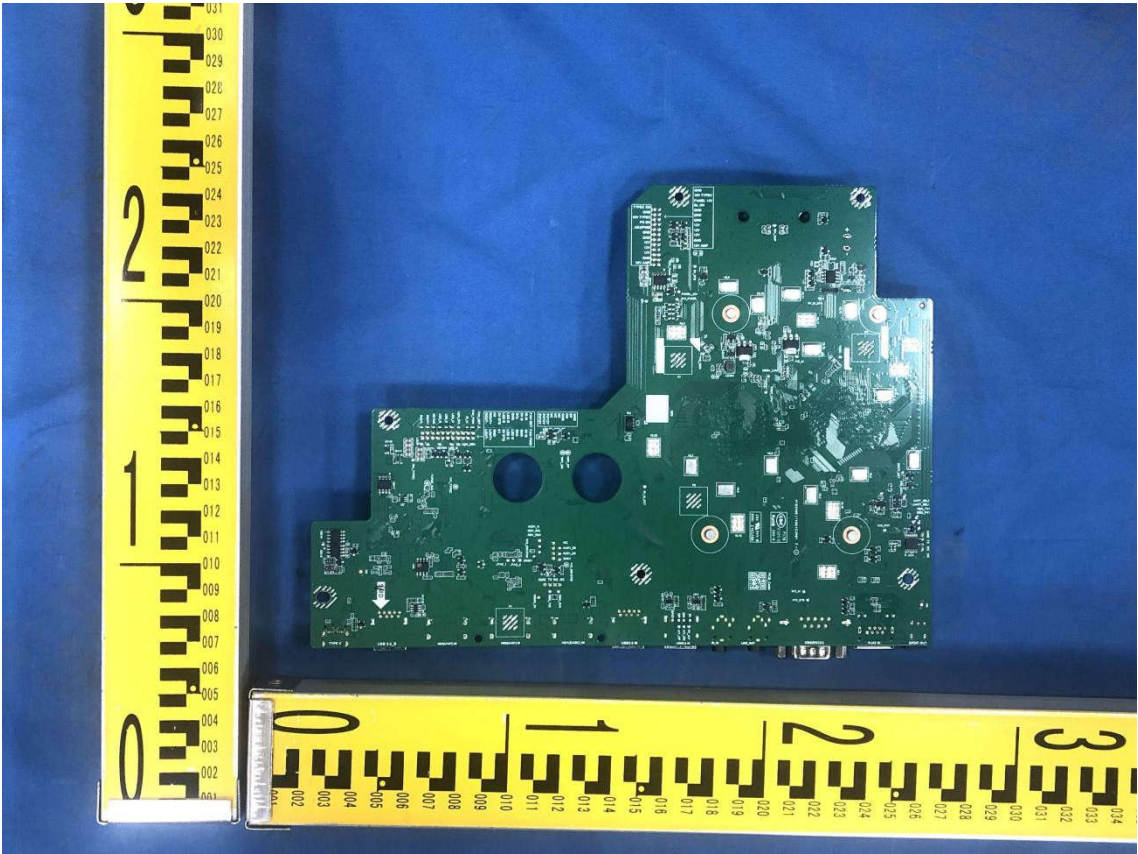
Figure 15. Main board T.MT9666.71 solder side view
