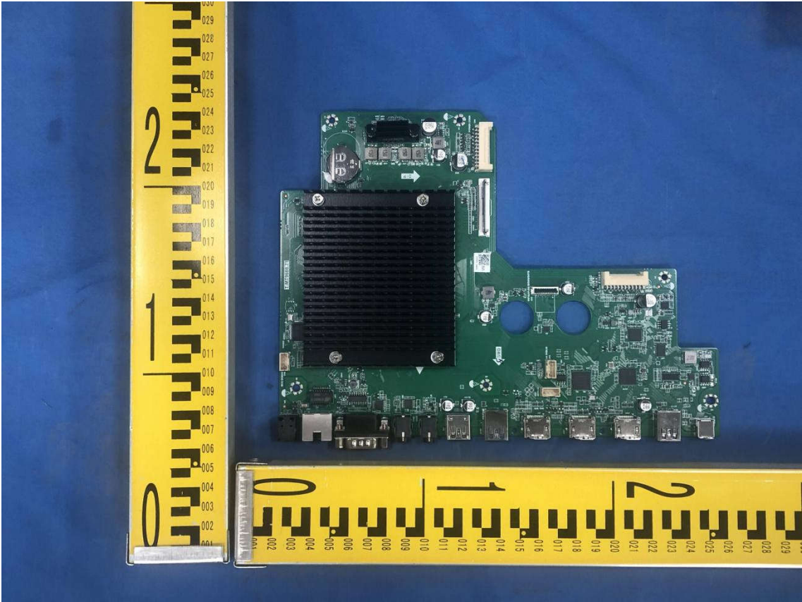
Figure 14. Main board T.MT9666.71 component side view
