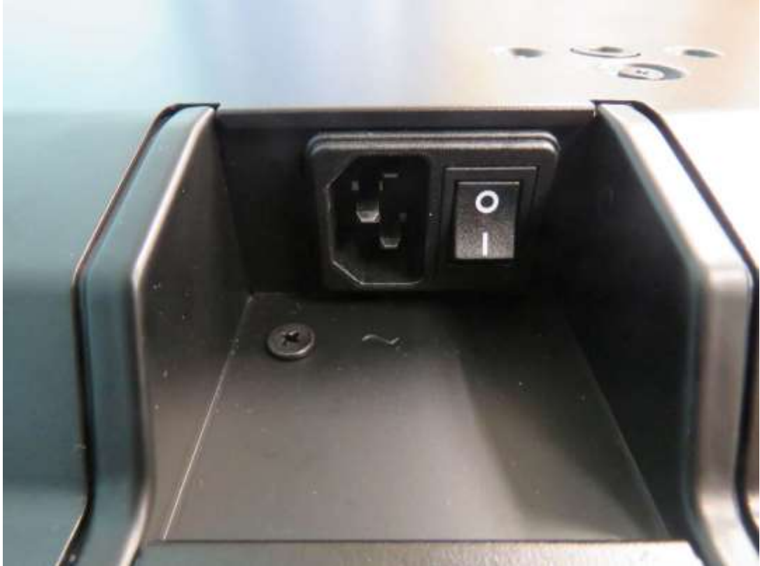
AC inlet and switch view
