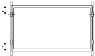
Fig. A2: Clamp position on short frames Mounting rails parallel to the shorter frame
