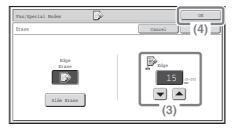
(3) Set the erasure width to 15 mm with the 🔽 🔺 keys.
