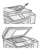
If the X dimension (width) of the document is less than 89 mm (3-1/2") or the Y dimension (height) is less than 100 mm (4"), place the original on the document glass.
