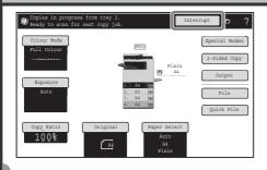
1 Touch the [Interrupt] key while the machine is printing.
