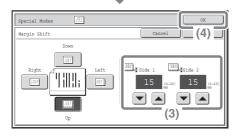
(3) Select 15 mm for the front side and 15 mm for the reverse side using the
